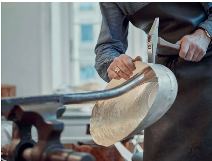
The Georg Jensen silversmithy does not use moulds. Instead, the hand-hammered half-egg shapes were measured periodically and refined until they reached the desired forms.
