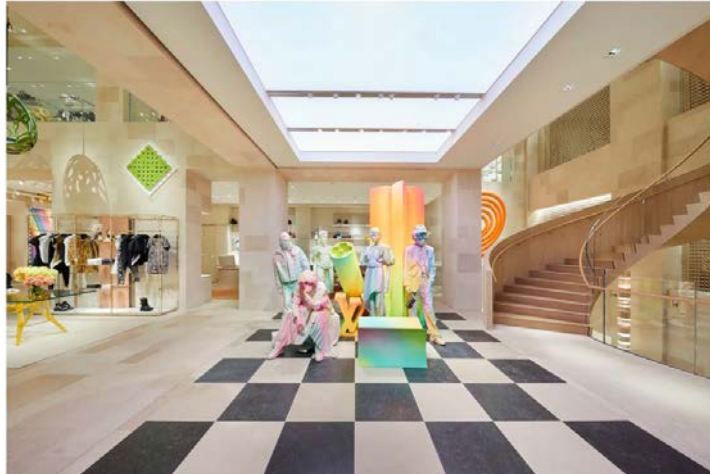
A chequerboard floor in a Damier check pattern, made of Croix Huyart French limestone and Pierre Bleue du Hainaut marble, greets customers as they enter the store. To the right, a staircase made of cerused oak guides the eye towards Josh Sperling's unnamed work and Chris Martin's Golden Age (for Harry Smith). Courtesy of Louis Vuitton
